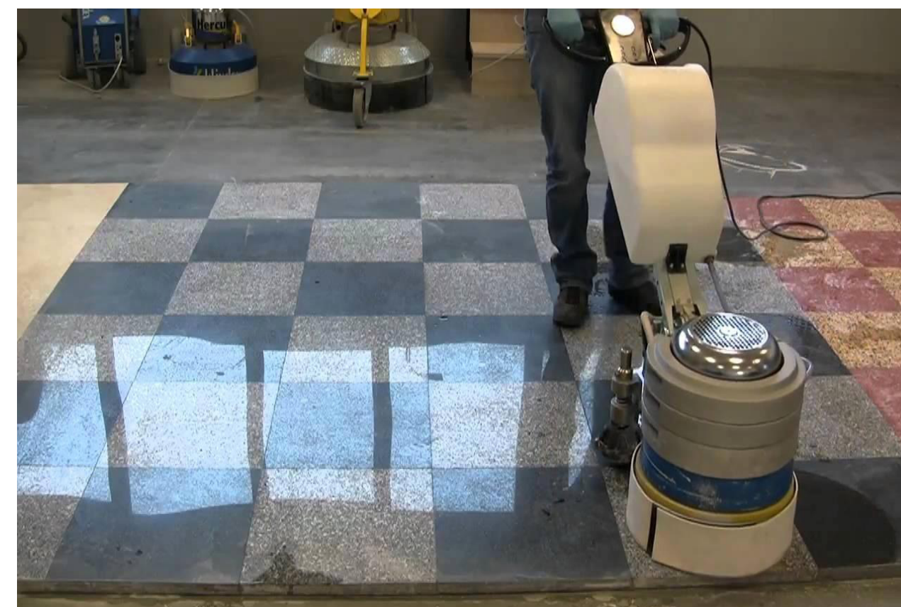
GRANITE POLISHING USING KLINDEX HIGH SPEED AND HEAVY DUTY MACHINE: MACHINE 150 KG GRINDING SPEED 2000 RPM
